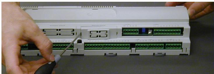
Fit the TREND system serial interface card (if not present) into the slot.
