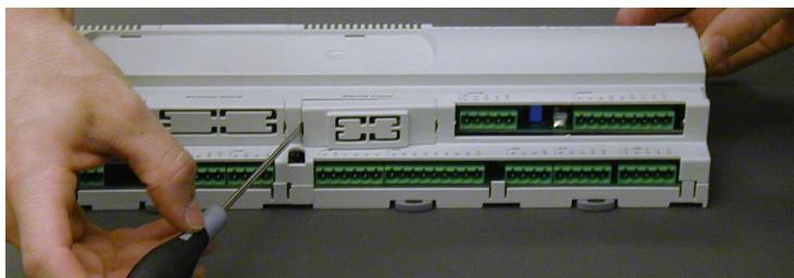
Fit the FWS serial interface card (if not present) into the slot.
