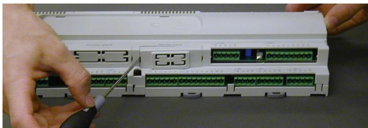
Fit the LONWORKS system serial interface card (if not present) into the slot.
