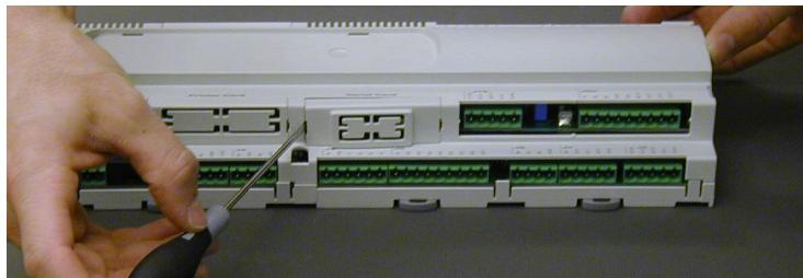
Fit the BMS serial interface card (if not present) into the slot.
